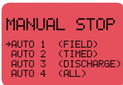
The user uses the UP and DOWN arrow keys to define a minimum field pressure that once achieved, will result in an auto start of the system. This value must be set above the LOW SUCTION PRESSURE setpoint. With the engine shutdown in STANDBY and configured in the AUTO 1 mode, the panel will RESET and initiate a start sequence if the Field Pressure rises to the FIELD PRESSURE TO START setpoint.
