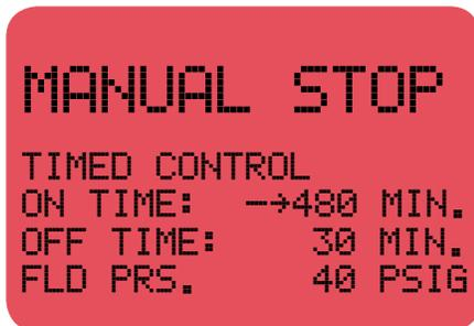
The times entered represent the number of minutes the system will run before shutting down, and the time it will remain shut down until it restarts. Refer to SECTION 29.0 for a detailed description of the start and shutdown sequence.
