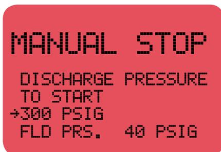
24.2 In this mode, the system will shut down if the discharge pressure exceeds the HIGH DISCHARGE PRESSURE setpoint. When the discharge drops below the DIS PRS (Discharge Pressure to Start) setpoint shown on this screen, the controller will RESET, open the VENT and BYPASS valves, and initiate a start sequence. Note that the DIS PRS value must be set below the HIGH DISCHARGE PRESSURE setpoint. Refer to SECTION 29.0 for a detailed description of the start and shutdown sequence.
