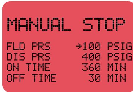
**NOTE:** The timer aspect of this mode can be disabled by setting the OFF time to zero.
